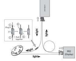
Please note: CD changer retention is not supported, therefore you need to disconnect it from the optical ring if present and loop the optical ring with the separate loop kit (FOA1TL1).
