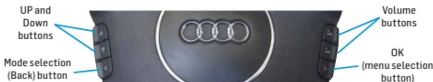
In case of this version of steering wheel controls, you can switch between media and phone screen with the (<) mode selection button. You can bring up the menu with the OK (>) button. To move in the menu you need to use the (▲) and (▼) buttons. You can enter menu and confirm selection with the OK (>) button and you can go back to the previous submenu with the Mode selection (<) button.
