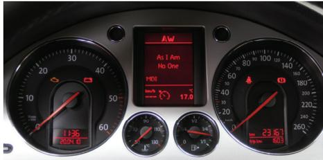
The menu of the iGateway is displayed on the car radio and partly on the central display on the dashboard (between the two main instruments).
