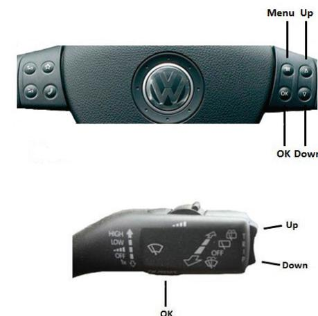
The menu can be selected and controlled from the steering wheel control or stalk control, whichever is available.
