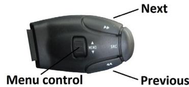
You can enter the iGateway main menu by pressing disc 6 on the Radio or by rolling the 'MEMO' wheel down on the stalk controller.
