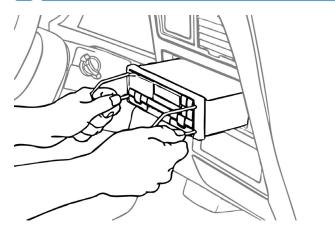
First, carefully remove your vehicle's existing OE head unit as per the factory instructions and using the correct tools.
