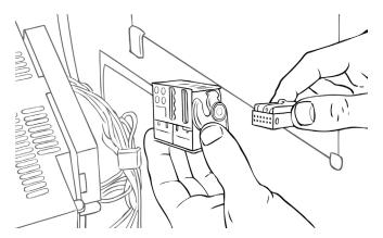
With the main radio cable removed, first connect the Dension supplied cable to the original factory cable harness.
