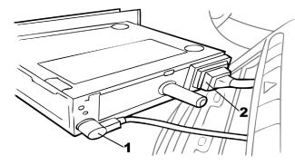
Once the head unit has been removed, disconnect the antenna cable (1), then unclip the main wiring connector from the head unit (2). This again, will differ in all makes and manufacturers.
