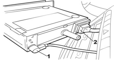
Once the main radio cable is removed, you can connect the Gateway with the supplied cable to the head unit. The connection methods may vary by each head unit versions, here are the possible situations:
