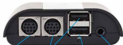
iPod Dock cable or cradle or DAB+G connector    Connector port (optional)    USB device    Microphone
