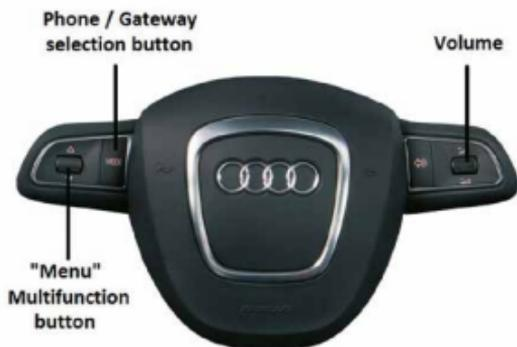
In case of the 6 button steering wheel controls, you need to use the next buttons.
