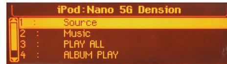
Toggling between different menu options is possible with the next (⏮) or previous track (⏭) buttons. In order to select a menu item, press and hold (about 3 seconds) the next track (⏮) button. You can get back to the previous menu level if you do the same procedure with previous back (⏭) button.
