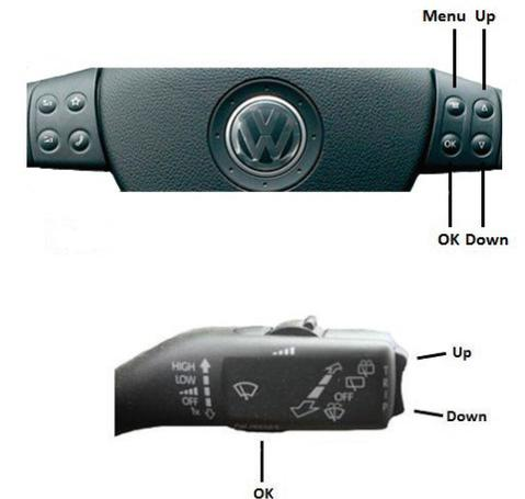
The menu can be selected and controlled from the steering wheel control or stalk control, whichever is available.
